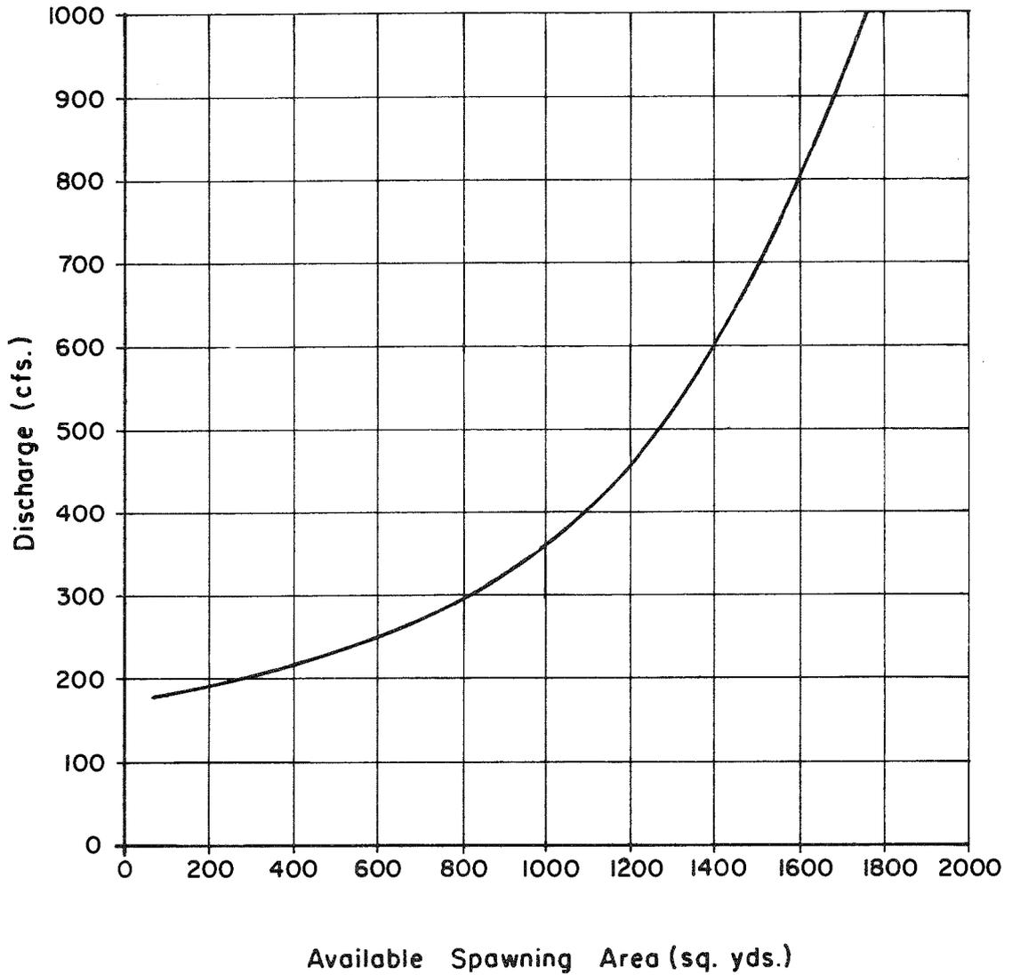
Figure 14. Nanika River - Relationship between spawning area and discharge, Spawning Area B.
