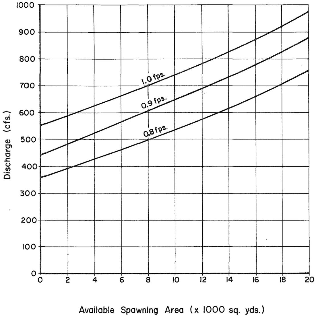
FIGURE 12. Nanika River - Relationship between available spawning area and discharge, Spawning Area. A.
