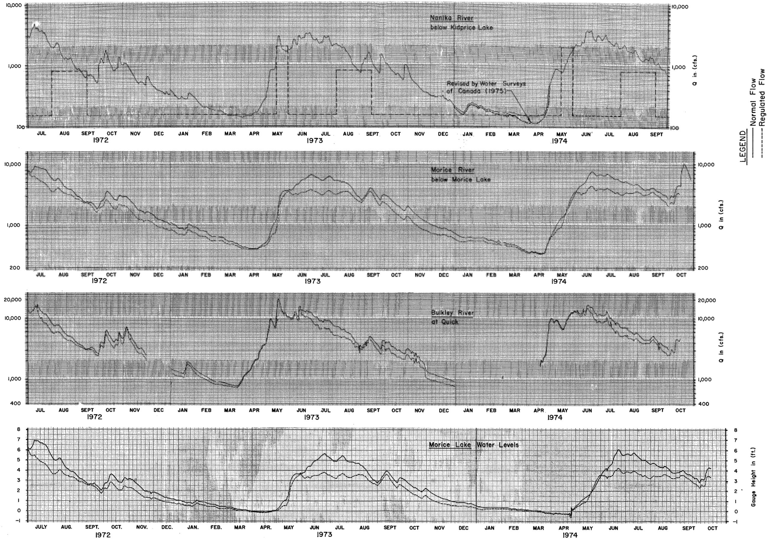
FIGURE 32. Hydrographs of natural and regulated discharges for Nanika, Morice, and Bulkley Rivers and water levels on Morice Lake, 1972 - 1974.
