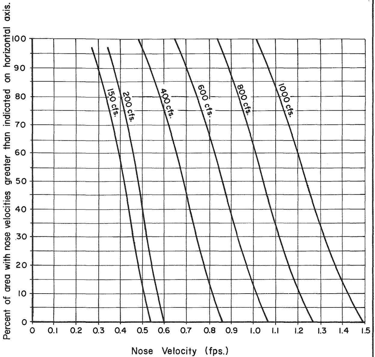
FIGURE II. Nanika River - Distribution of nose velocities for various discharges, Spawning Area A.
