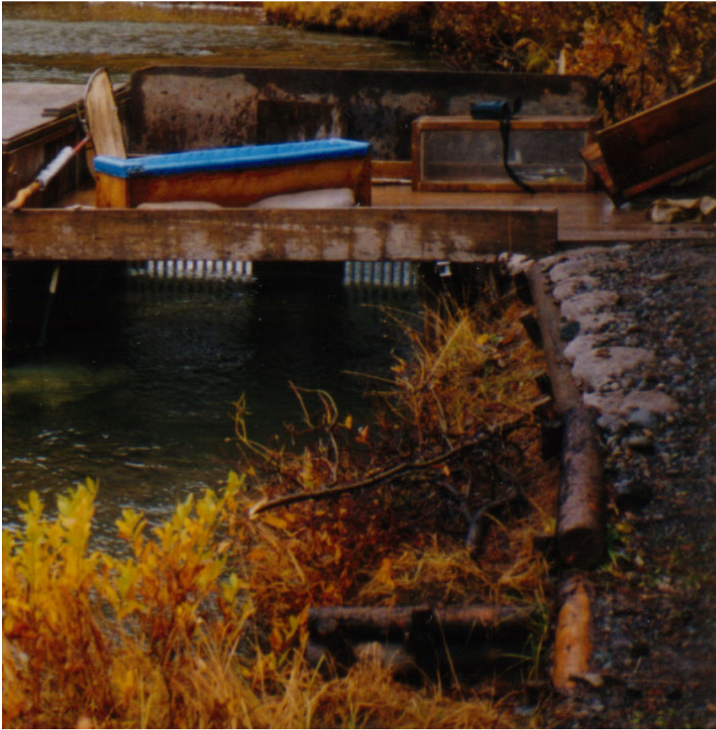
Photo Figure 9. View of the right bank looking downstream towards the trap box deck. Note a) the blue foam lined measuring tray; b) the viewing box (top right); c) efforts to improve bank stabilisation around the fence working areas.
