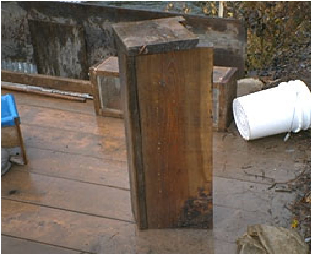
Photo Figure 7. View of trap box shroud sitting on top of the fence work deck. Note the acrylic bottomed viewing box behind the shroud.
