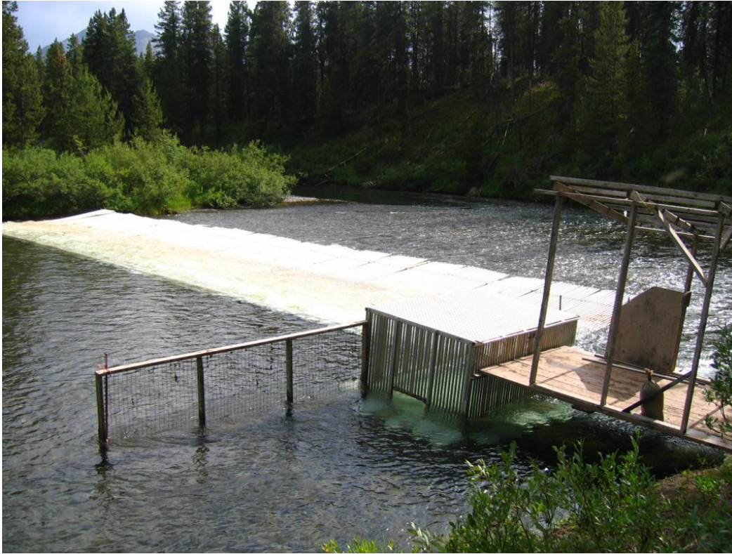
Figure 3. Upper Sustut steelhead enumeration fence, trap box and sampling location. Photo courtesy of Brome and Leaf Steffey.
