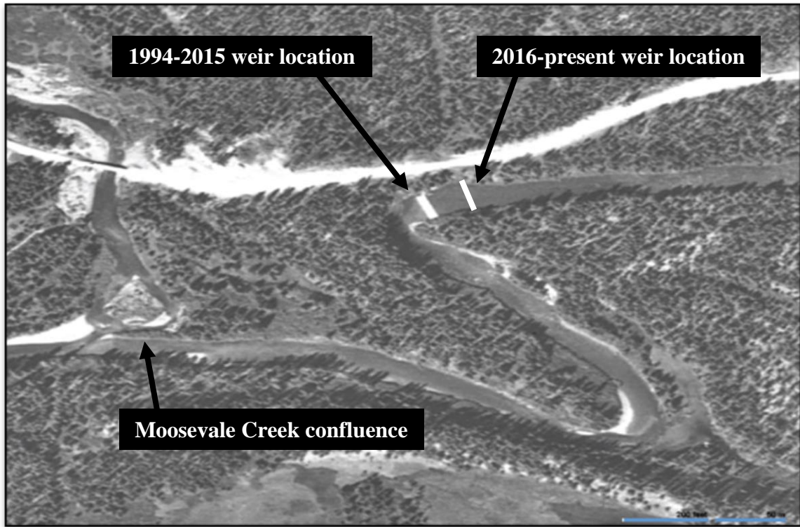
Figure 3. Aerial view of Sustut enumeration weir relocation
