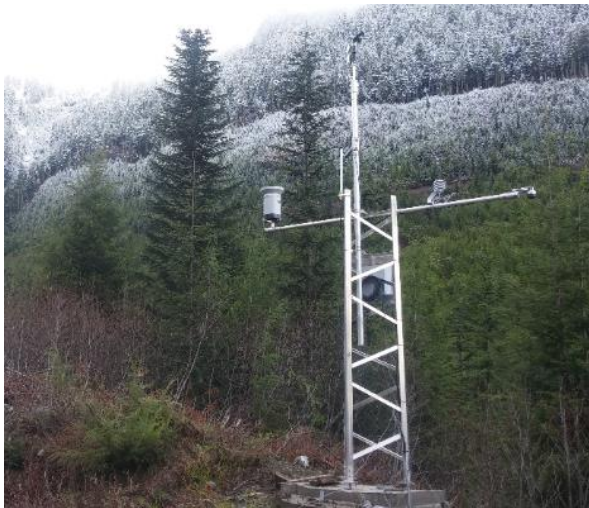
Figure 2. Example of a climate station equipped with real-time transmitting capability (Russel Creek, BC). A similar station will be installed in the Stein watershed to track climate variables alongside hydrological attributes.
