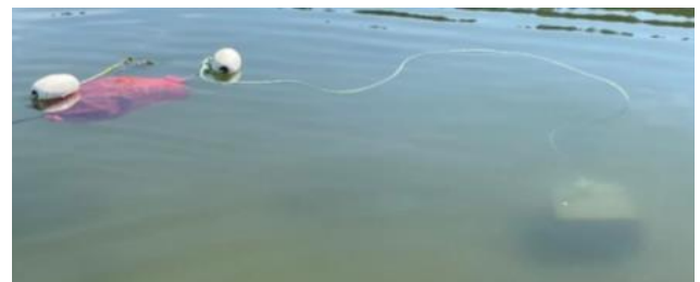
Figure 1. BuDS set: anchor, floating line, and 2 buoys with net bag of reproductive shoots clipped to the line.
