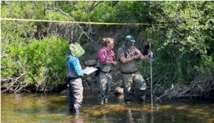
Figure 1. Flow transect acquired at the time of level logger installation on July 17, 2024.
