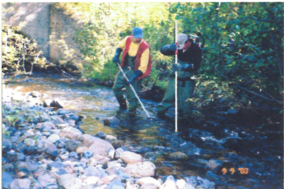
Fig.3 Upstream baseline sampling using a Smith-Root 12B POW backpack electroshocker and dipnet.
