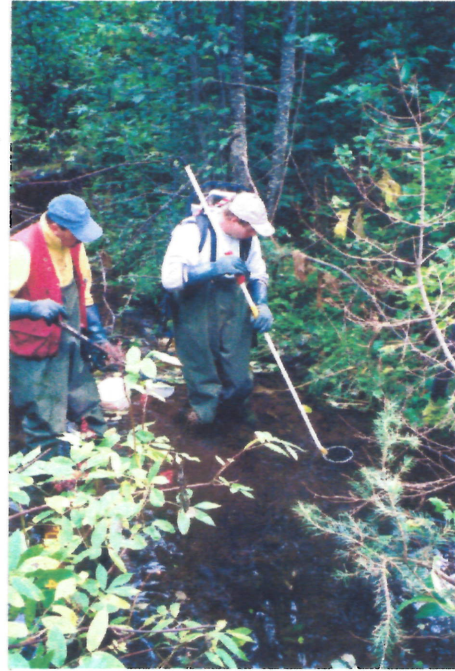
Fig.1 Fish salvage using a Smith-Root 12B POW backpack electroshocker.
