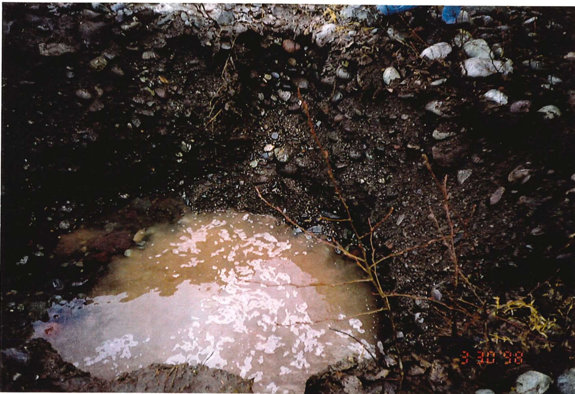
Photo 7: Sub-surface water reached at 1.5 m in test hole one.
