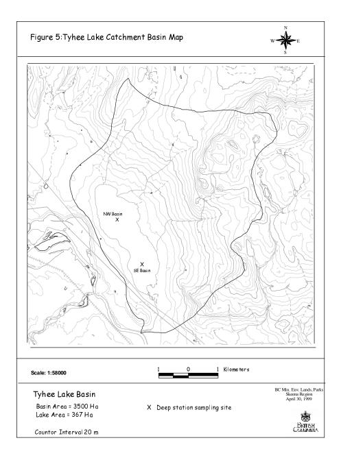
Tyhee Lake is in the Skeena watershed and the catchment basin is outlined in Figure 5 (Skeena GIS, 1995). The approximate size of the catchment basin is  $35 \text{ km}^2$  (3500 ha). The catchment basin is determined by the physical height of the land and the boundary outlines the area within which all water flows towards the lake.
