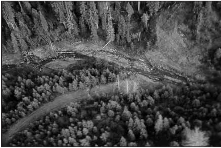
Figure 6-10. Aerial view of Site 3. Note high quality second growth for future long-term recruitment of LWD. To address short-term LWD deficiencies logs were placed parallel to the stream flow to encourage bank and mid-channel bar stabilization.
