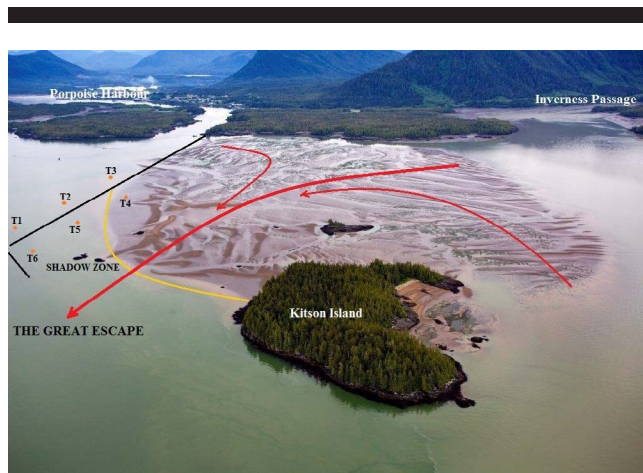
Figure 20. Based on the interpretation provided by the STA, it is predicted that sand will be lost from Flora Bank (the Great Escape) following construction of the trestle portion of the terminal jetty. Because the energy of the processes affecting Flora Bank will be reduced between the start of the trestle and Kitson Island (the shadow zone), inequality of the energy between the two sides of the bank will allow sand waves to advance, causing a seaward loss of sand in the approximate directions of the red arrows. T_1 to T_6 are the approximate locations where current velocities have been modeled before and after trestle emplacement (discussed in text).
