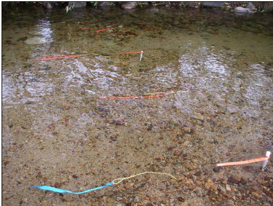
Photo 4. Completed installation of piezometers and buried incubation cassettes, flagged with poly rope and tape to facilitate locating for incubation assessments, at Site 4 in Scully Creek mid channel.
