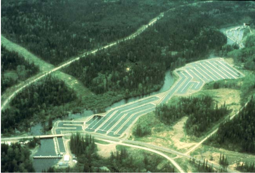
Fulton River Spawning Channel #2 and Counting Fence. Channel No. 1 in the background requires rehabilitation as egg to fry survival has dropped to about 15%.
