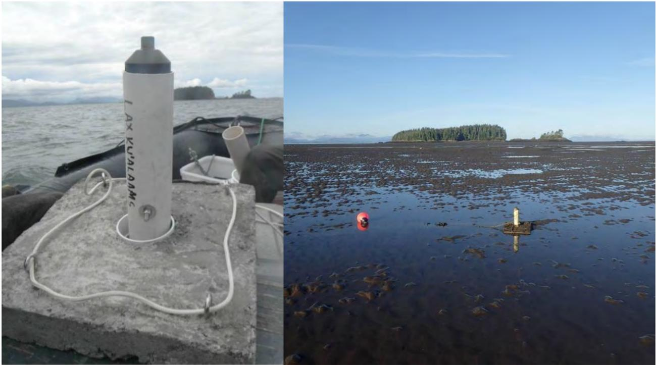
**Figure 5-24.** A stationary acoustic receiver/logger with its concrete pad and PVC tubing assembly (left) and installation on Flora Bank during low tide (right).
