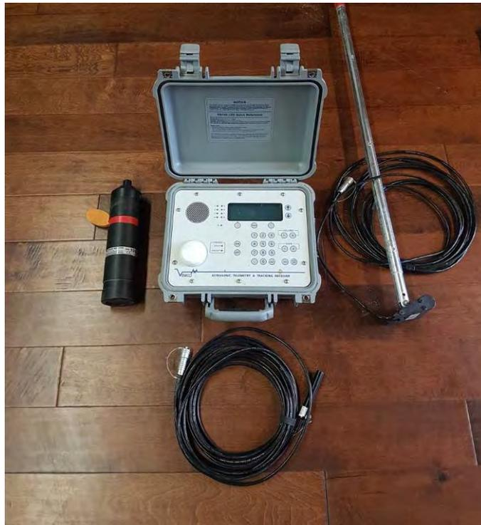
**Figure 5-23.** Acoustic telemetry tracking equipment used in the 2016 Dungeness crab study: Vemco VR2W stationary receiver/logger (left), Vemco VR100 acoustic receiver (center), pole mounted Vemco VH110 directional hydrophone (right), and Vemco VH165 omni-directional hydrophone (bottom).
