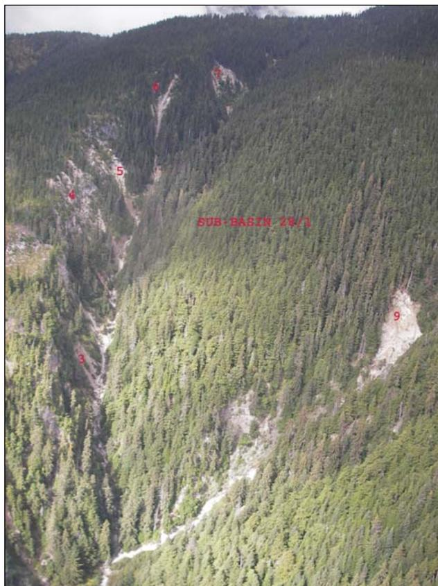
Figure 4-5. Actively failing gully sidewalls in subbasin 28/1.
