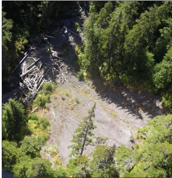
Figure 4-15. Subbasin 40, site #40-51. Stream side escarpment failure in glacial till.
