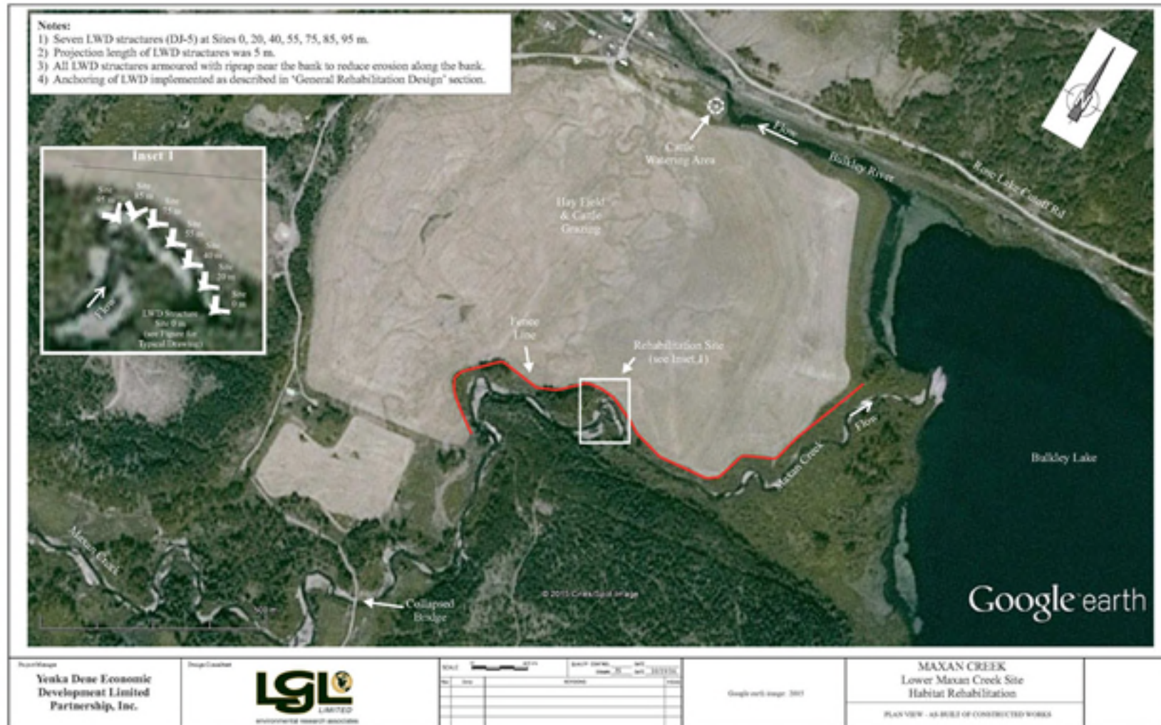
Figure 5. As-built plan view of rehabilitation works at the lower Maxan Creek site.
