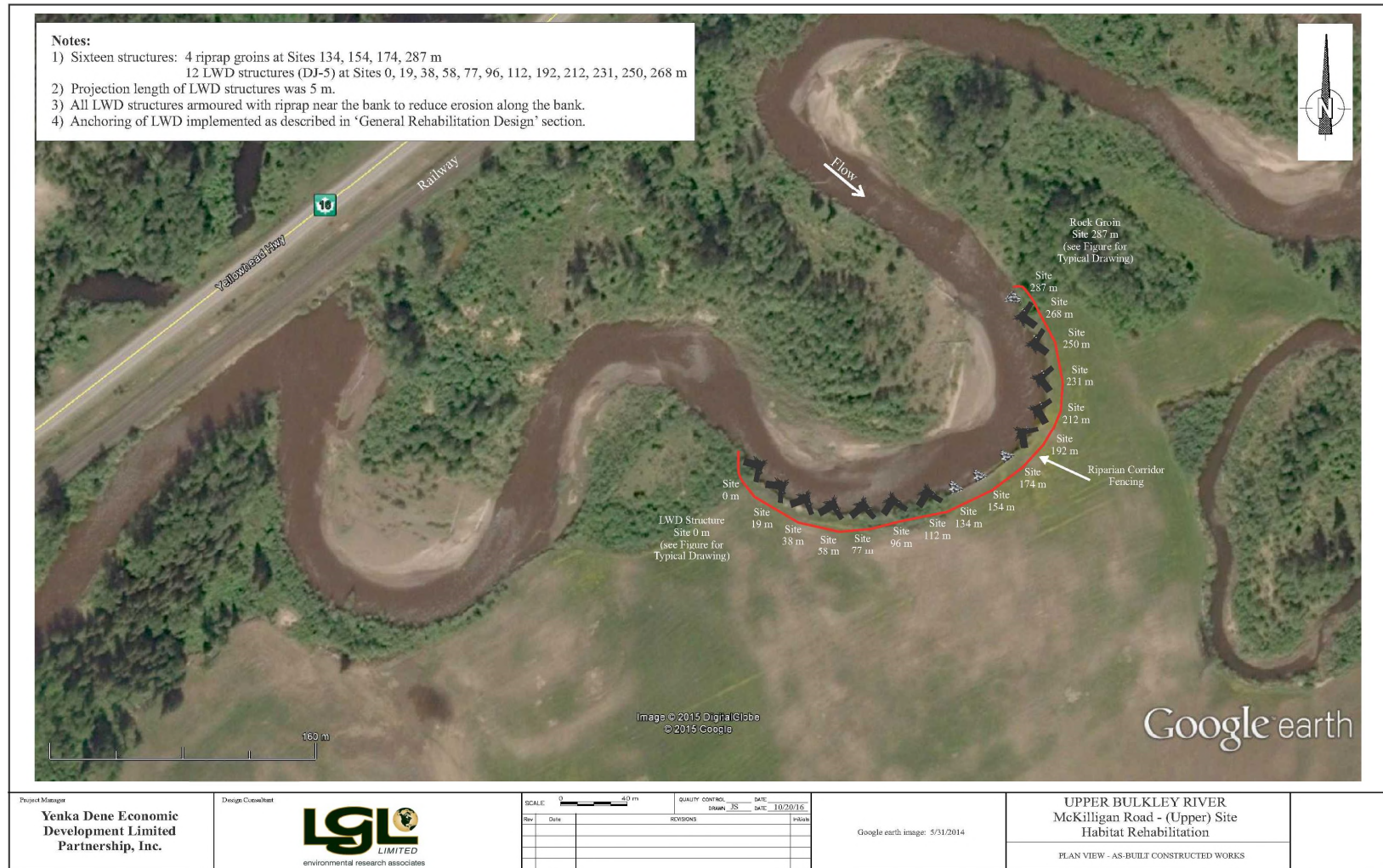
Figure 7. As-built plan view of rehabilitation works at the McKilligan Road (Upper) site on the upper Bulkley River.
