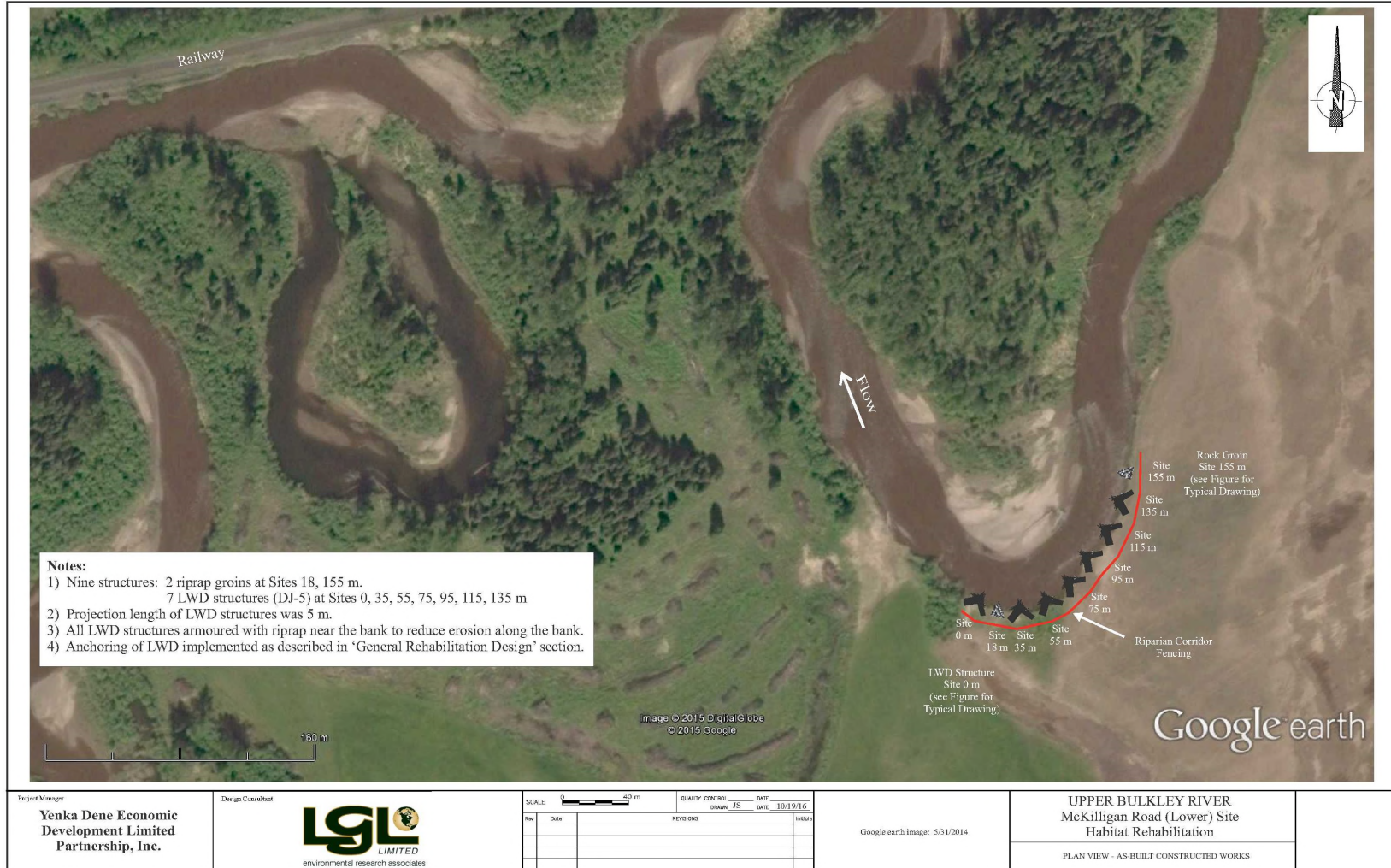
Figure 8. As-built plan view of rehabilitation works at the McKillingan Road (Lower) site on the upper Bulkley River.
