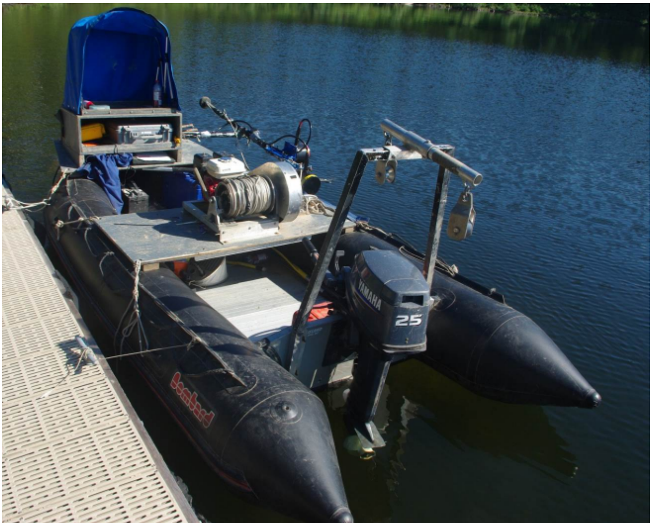
Figure 2. Photo of the inflatable vessel with the hydroacoustic gear.
