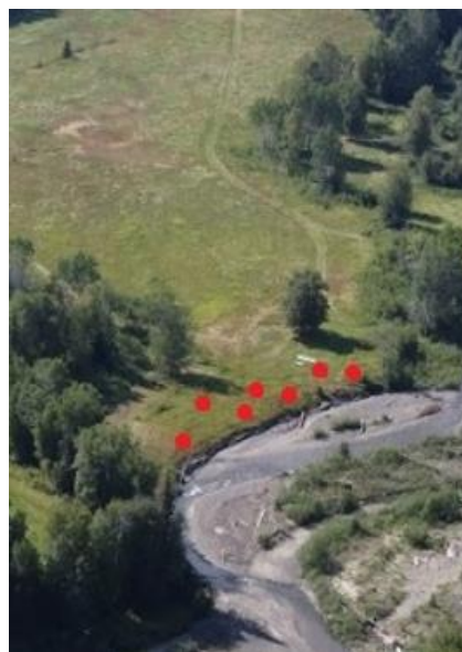
Figure 6. This image illustrates the section of bank which was planted with two rows of spruce seedlings (80 total). The seedlings were planted to prevent bank erosion/land loss.
