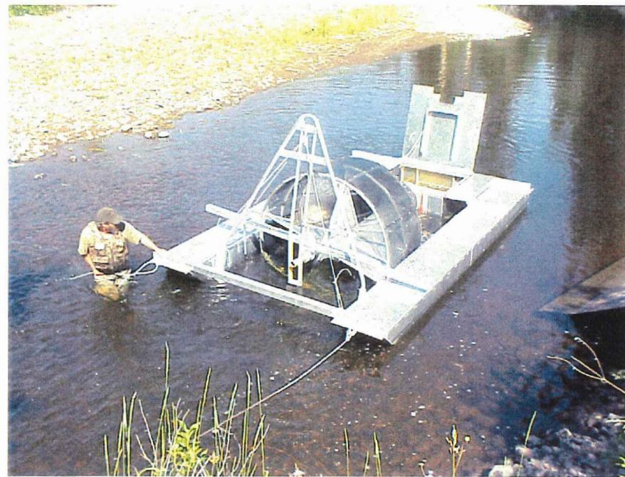
Figure 2: Maneuvering the 6 foot rotary screw trap into place at the head of a pool (above).
