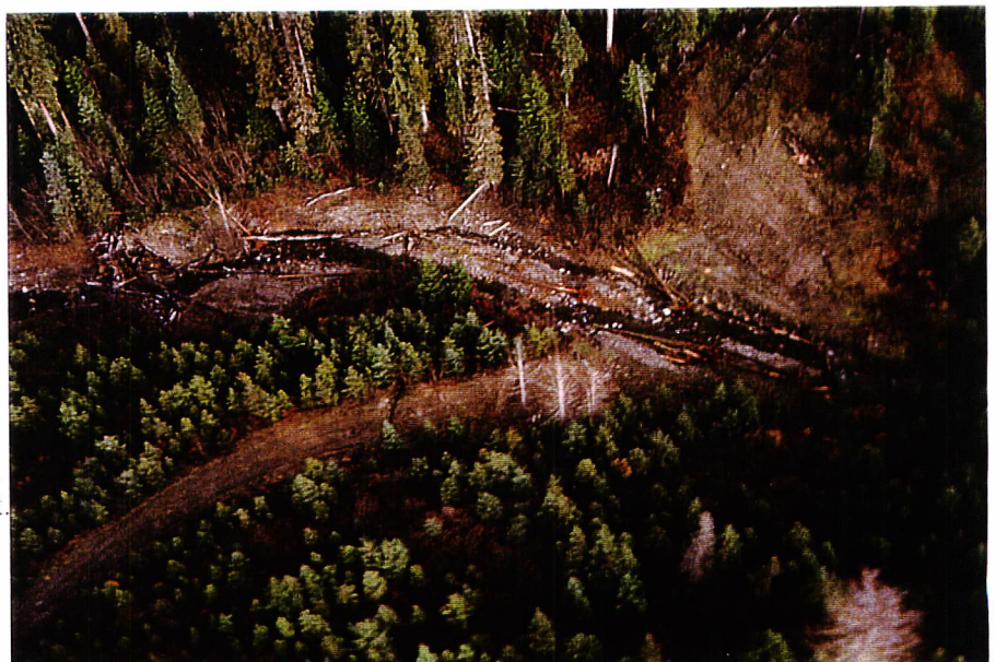
Photo 3 looking upstream after pullback of the collapsed bridge. The foreground shows a thalweg formed around a collapsed bridge structure removed during 1997. The sediment wedge in the upper right of the photo was deposited above the bridge in a 1 in 100 year event and is considered stable.
