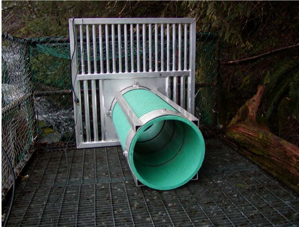
Picture 1. Kloiya River resistivity counter tube
