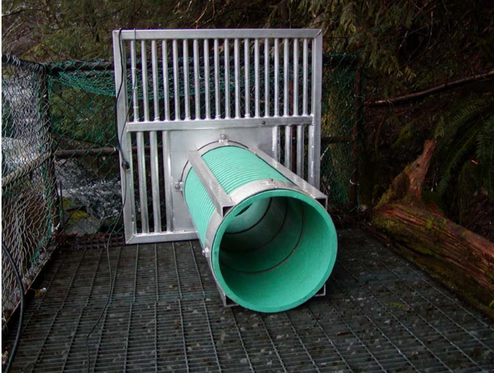
Picture 1. Kloiya River resistivity counter tube.
