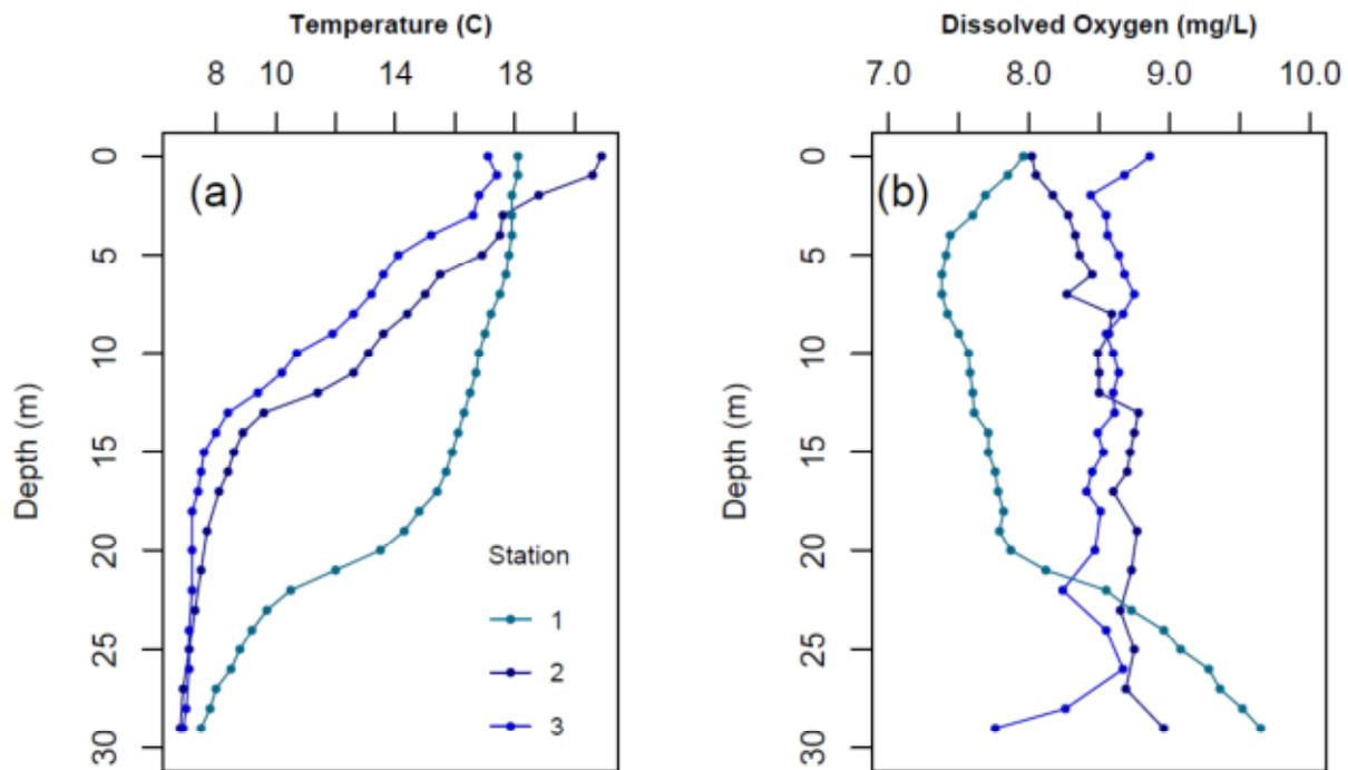
**Figure 5.** (a) Temperature and (b) dissolved oxygen profiles recorded at North Arm of Babine Lake, on September 9, 2015 (Station 1), September 10 (Station 2), and September 11 (Station 3)
