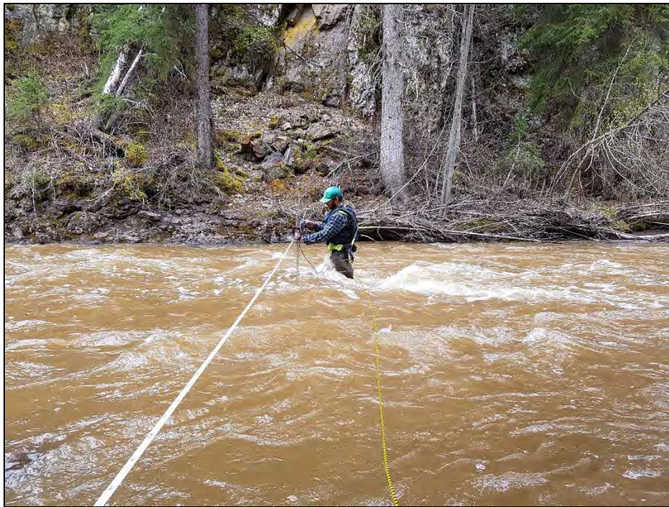
Plate 7.4-4. Velocity-area discharge measurement on Goathorn Creek. May 17, 2017.
