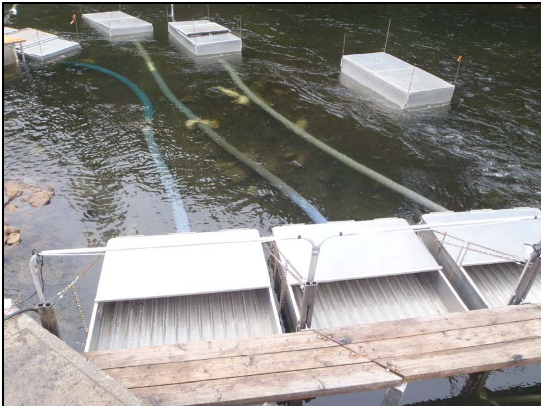
Figure 2: Photo of smolt trap box showing dewatering screen.
