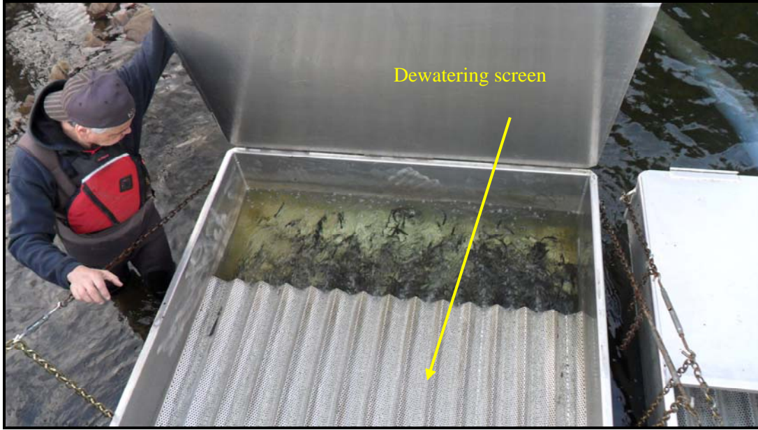
Figure 2: Photo of smolt trap box showing dewatering screen.
