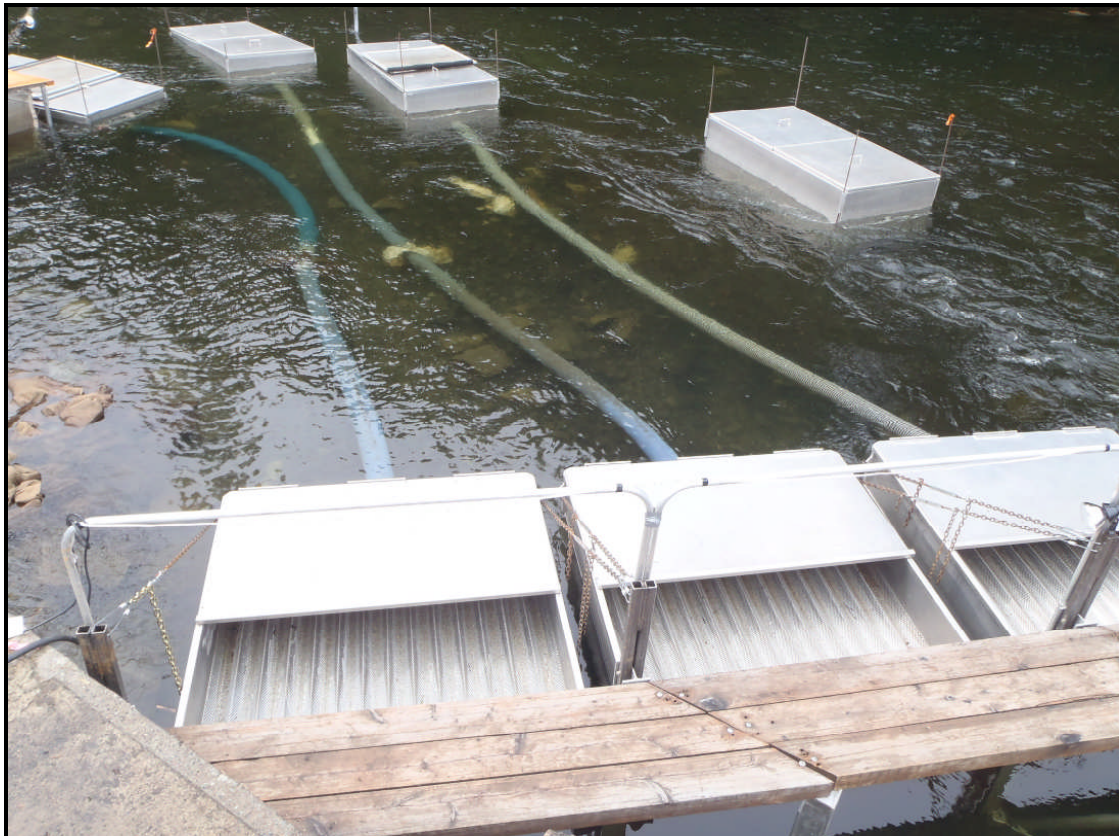
Photograph 2. Large holding boxes attached to smolt trap boxes with 6" hose.
