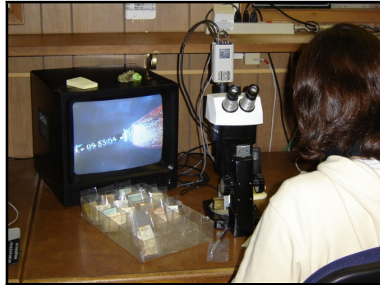
Figure 7: Figure 8: Photo of CWT being extracted from salmon head (left) and CWT read under microscope (right) - http://www.rmpec.org/recovery-gallery.html#
