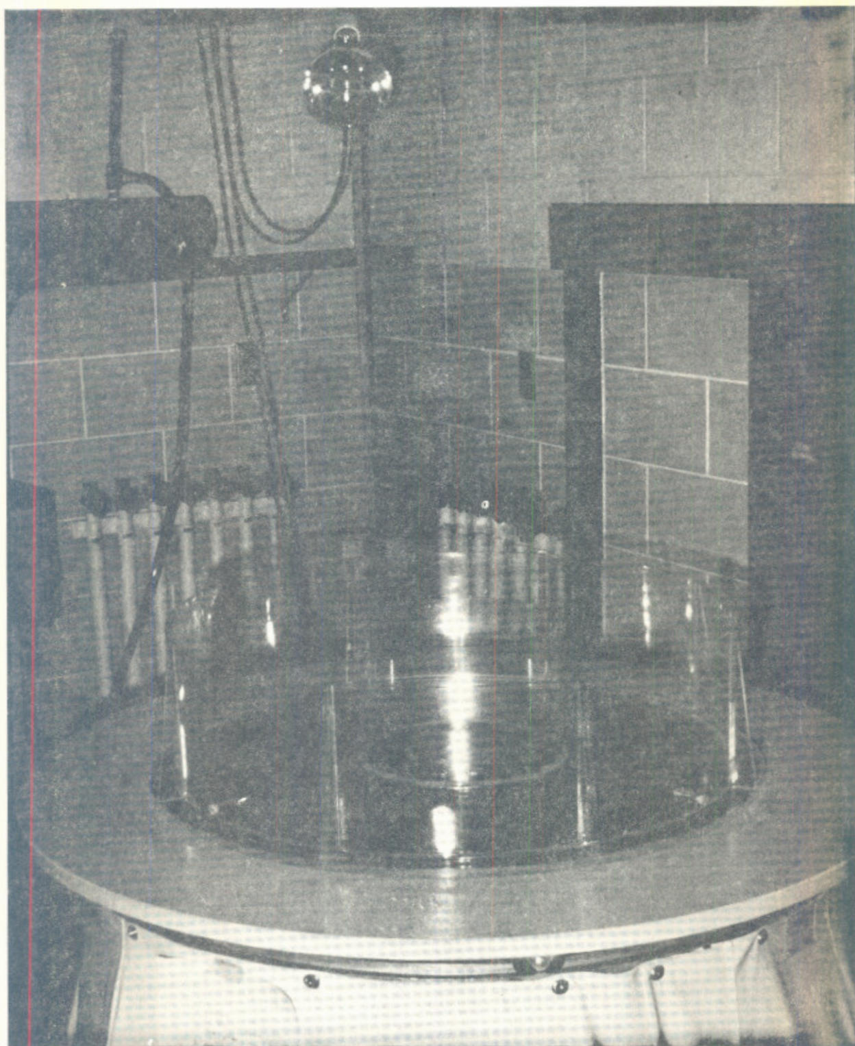
Fig. 5. Indoor test apparatus without tank cover. A fish was placed in the clear acrylic drum tank in the center. The lamp in the background is the artificial sun. Approximate scale: 1:10.
