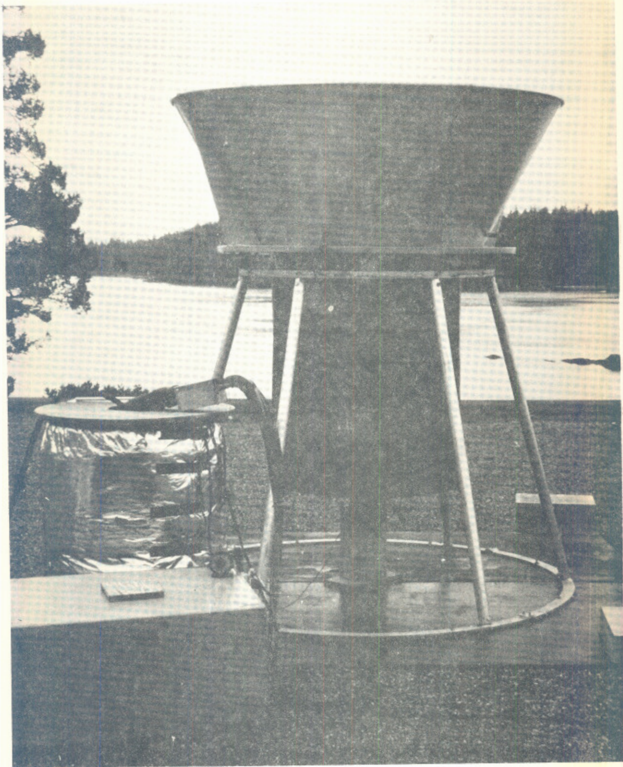
Fig. 2. Outdoor test apparatus on the roof of the F.R.B.C. Pacific Biological Station. The canvas cover which enclosed the base of the tank has been removed to show the plastic curtain shield and camera mounting. Approximate scale: 1:30.
