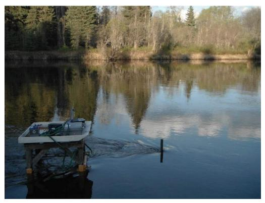
**Figure 5.** Photo of the hydroacoustic system collecting side-looking acoustic data from the river's left shore. May 25, 2014.
