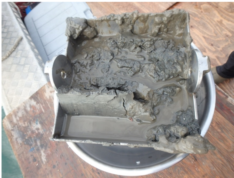
Photo 1 Surface Grab Sample Collection with a Shipek Sampler (Site SS04 at Berth 2)
