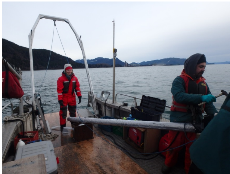
Photo 3 Vibracore Drilling System used to Collect Shallow Core Samples, with A-frame used for Maneuvering Vibracore System
