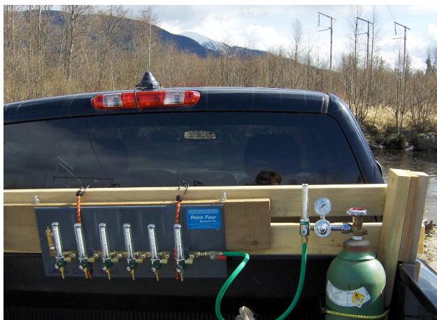
Figure 9. – Field Air Supply and Manifold
