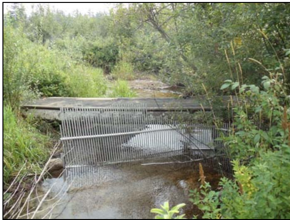
Photo 8. Scully broomstick fence with camera box.
