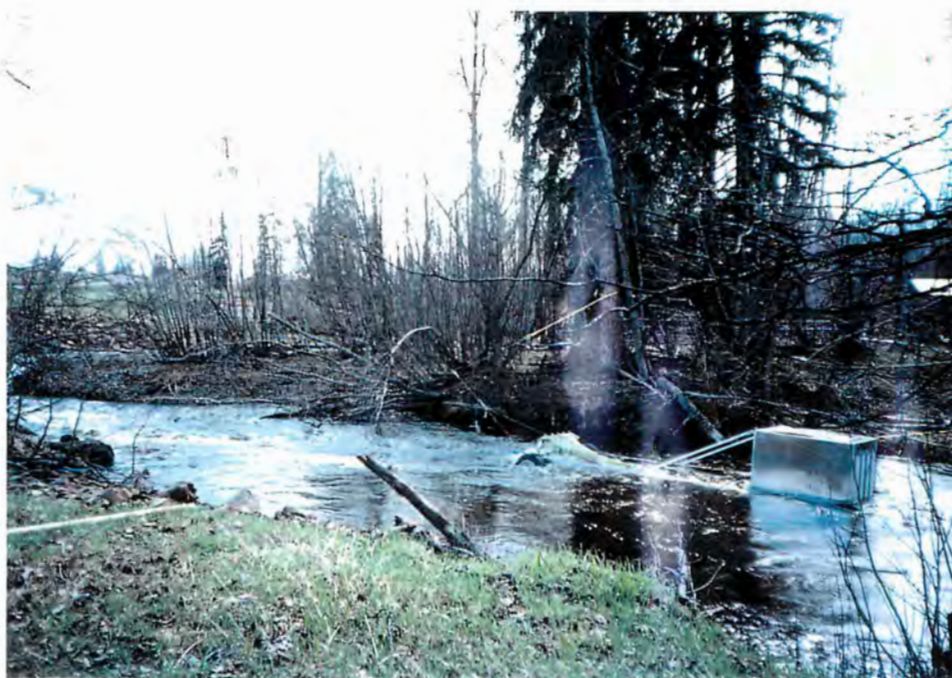
Figure 2. Example of common Fyke net setting at Toboggan Creek in the spring of 1996. Note trap position which provided good trap performance by intercepting high velocity water.
