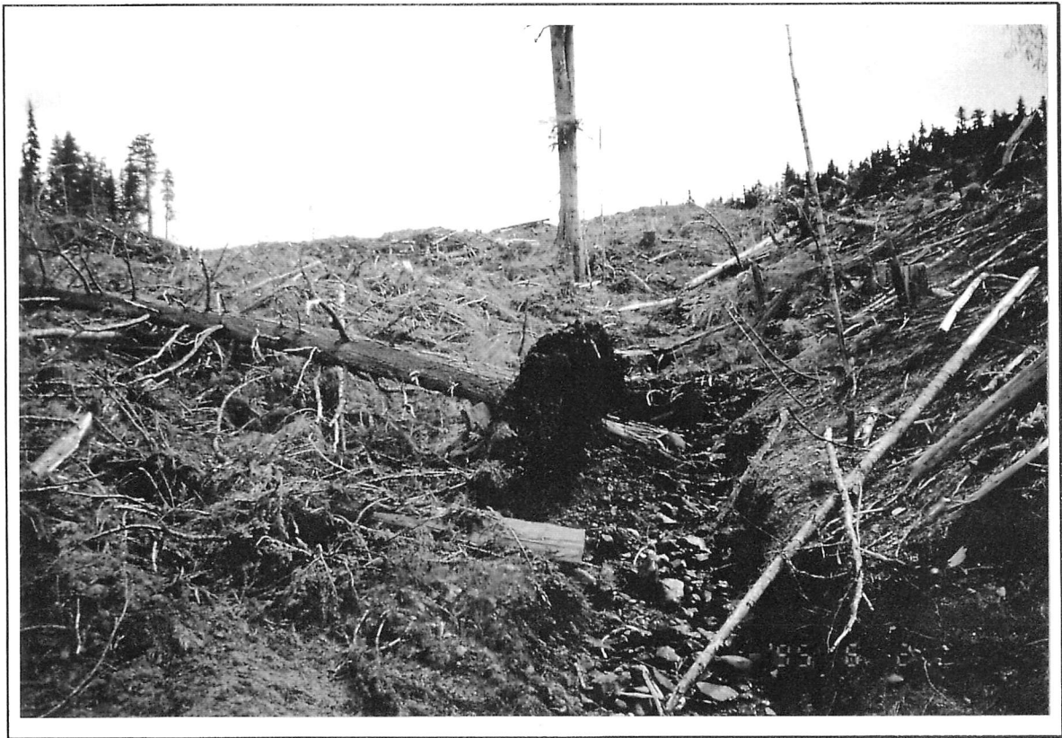
Figure 3.1) The terrain above is considered to be of very low concern to logging and road building operations. With a low (L) surface erosion potential and terrain stability classes II (interpreted using terrain stability and surface erosion potential map 93L.081 (Maynard 1994)), this terrain is considered to be a green zone where development may safely proceed. As seen above, slight problems of erosion from disturbed soils are to be expected in these zones. Periodic inspections of green zones and appropriate erosion control measures (such as grass seeding) may therefore be needed (D. Wilford, personal communication, August 1995). This photograph was taken from the McDonnell Main Road approximately 2 km south of the Moore Creek crossing.
