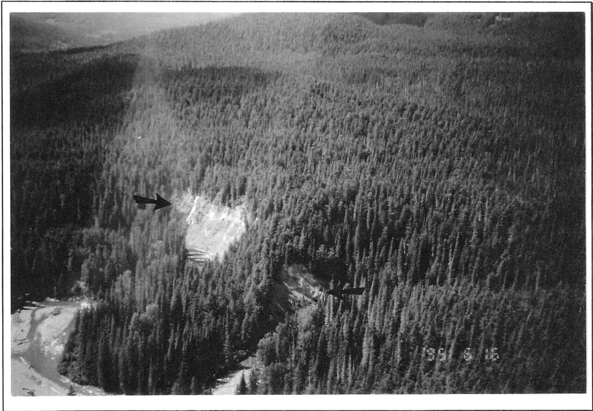
Figure 3.5) In the picture above, rapid erosion occurs naturally less than a kilometre from where Mulwain Creek enters the Zymoetz River. Rated by Denny Maynard as terrain stability class V with very high (VH) surface erosion potential (1994, Map 93L.071), the actively unstable terrain is considered a red zone to forestry development. No road construction or timber harvesting of any kind should take place in these actively unstable red zones unless approved by a qualified terrain specialist after careful field evaluation.
