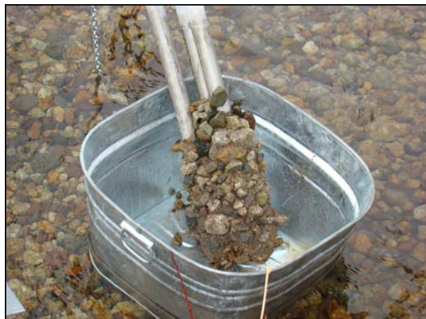
Photo 18 – Size of sample collected using the larger pipes and triple probe system.
