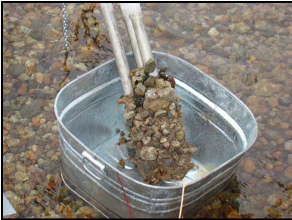
Photo 7 - Scully Creek - freeze core sampler with intact sample frozen to probe.
