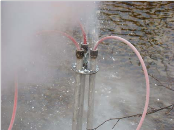
Photo 15 – (custom) Freeze core sampler in operation
