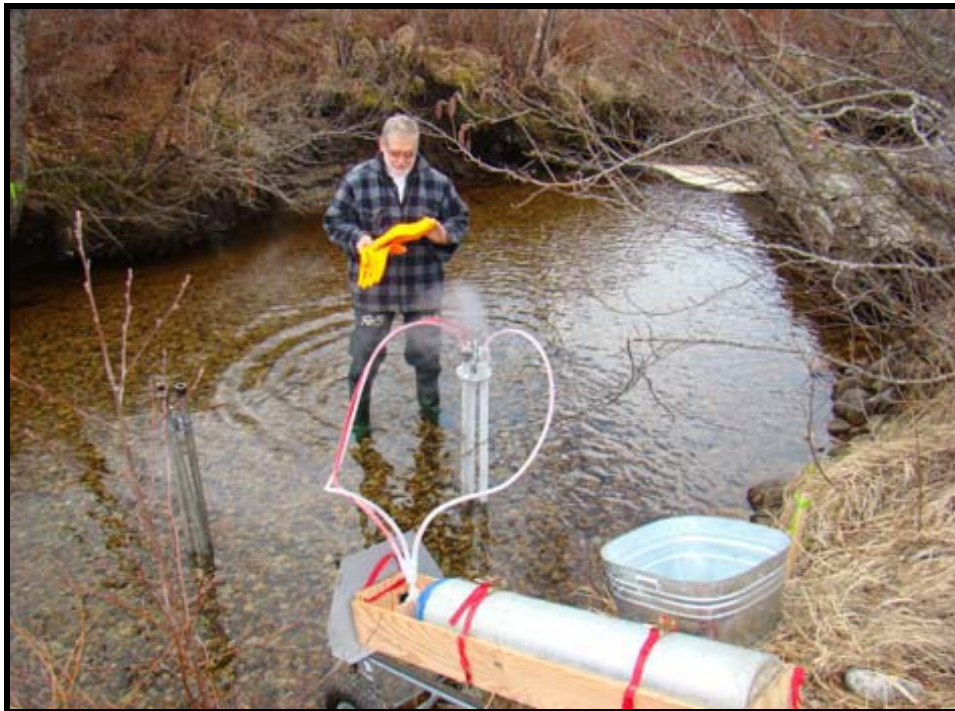
Photo 6 - Scully Creek - freeze core sampler at one of the spawning platforms.
