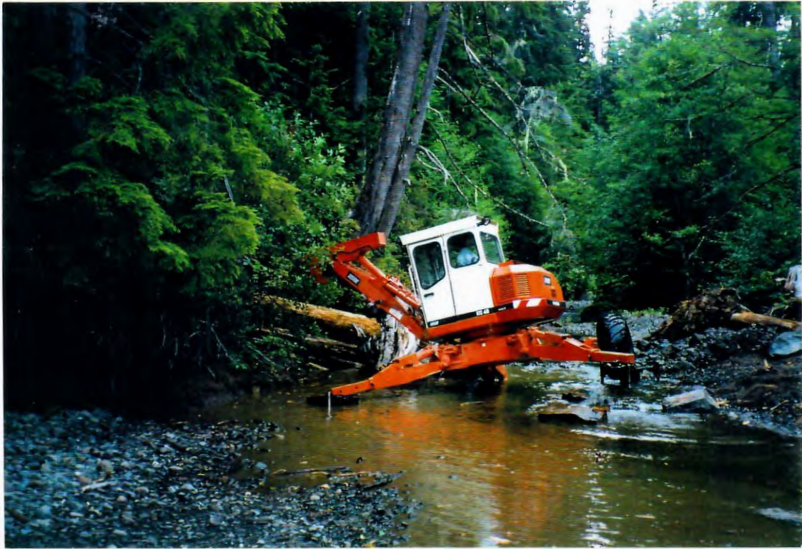
Photos 23 & 24. The Schaeff Superhoe™ spider is highly functional and versatile for instream work.
