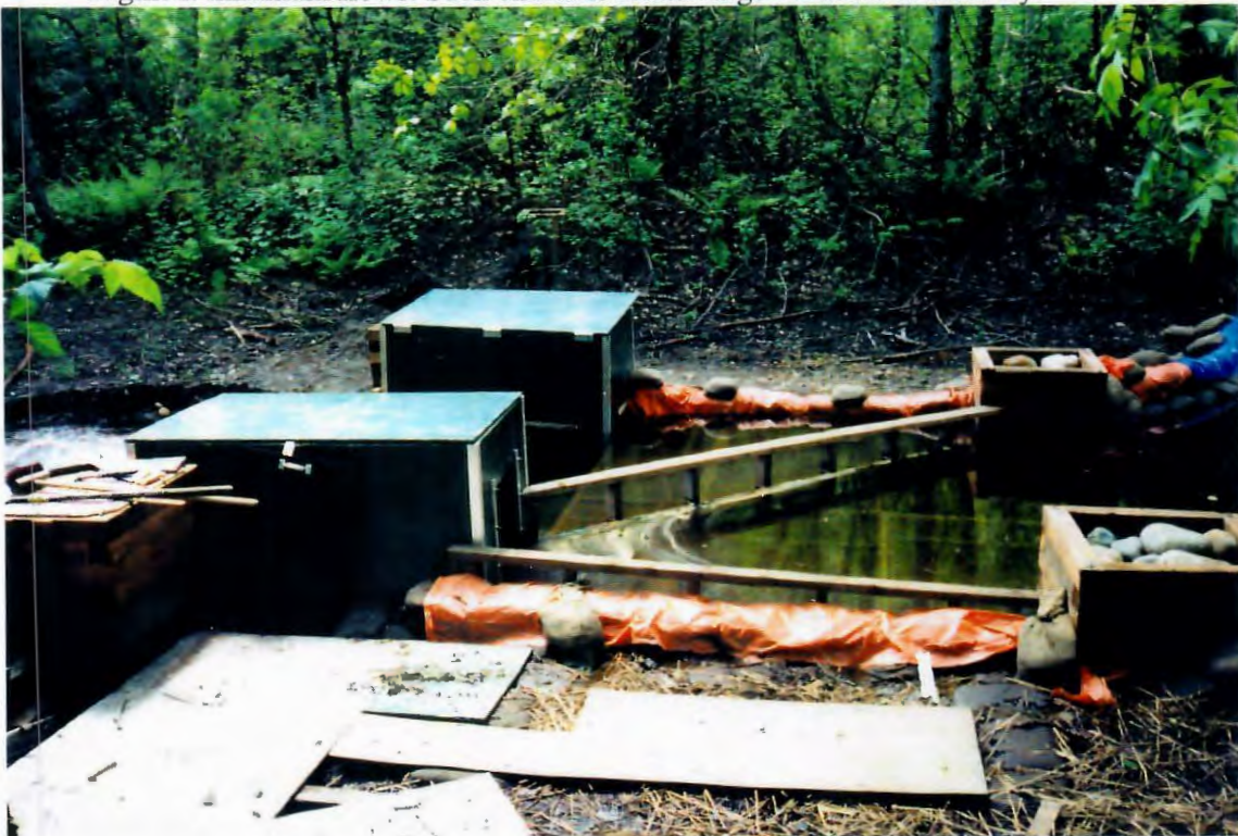
Photo 13. Horizontal screen trap. In 1996, 26% of coho smolts produced from Shop Creek (7150 in total) originated from two constructed groundwater channels and the overwintering pond.
