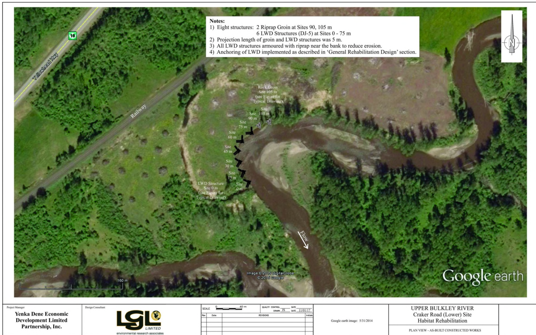
Figure 5. As-built plan view of restoration works at the Craker Road (Lower) site on the upper Bulkley River, 2017.
