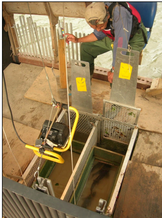
Photo 3: GFA technician identifying and counting salmon at one of the two trapbox locations on the KSEF. Note the green boxes inside the trapboxes, which have plexiglass bottoms. Fish swim overtop a white teflon surface making identification easier.
