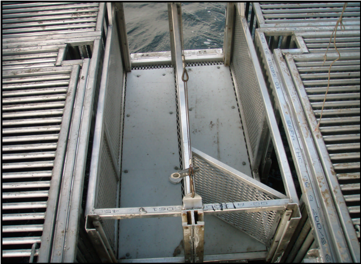
Photograph 4. Left bank trap box.
