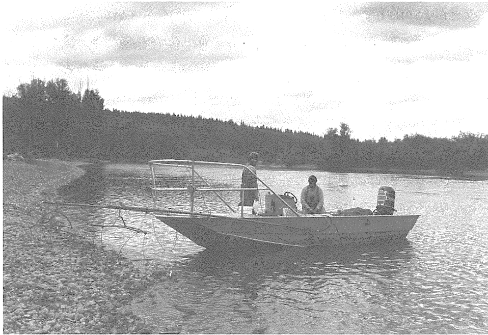
Plate 1: River boat modified for electrofishing. Note adjustable anodes on the bow.
