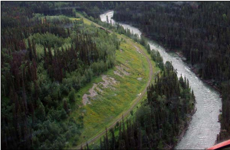
Figure 33. Sustut River with minor cutslope erosion 30 years later, 2007.
