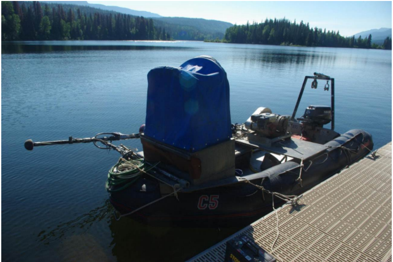
Figure 2. Photo of the inflatable vessel with the hydroacoustic gear.
