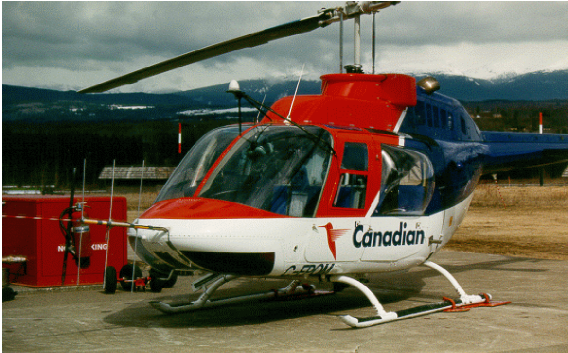
Figure 5. Helicopter used for tracking flights showing the location of telemetry antenna, mounted on the aircraft's high frequency antenna, and GPS antenna (white dome over front window).
