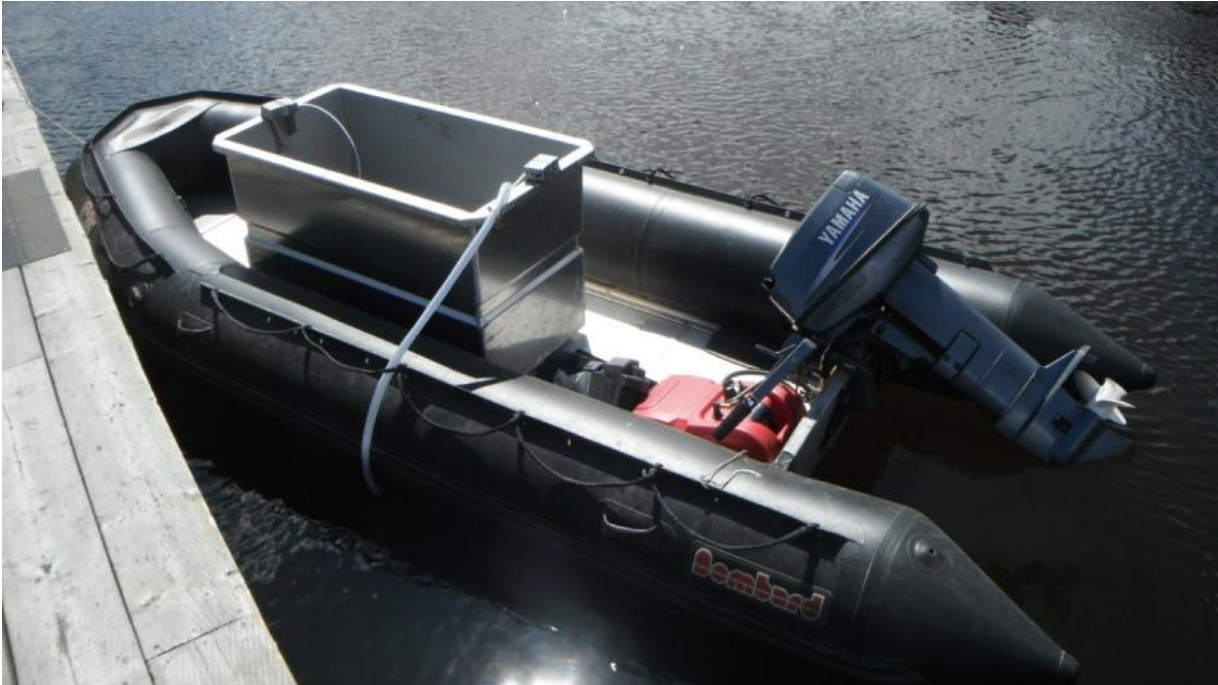
Figure 7. View of the inflatable boat used to release tagged sockeye smolts at the south end of Nilkitkwa Lake. The metal tank was filled with water and held over 3,000 tagged sockeye smolts for transportation.
